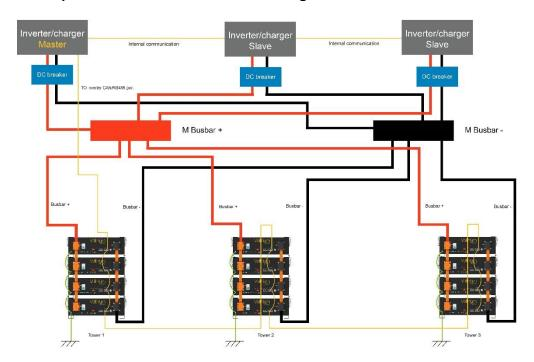
Considering system stability, when you install multiple batteries, please always keep a certain capacity margin of 30~50%. it is recommended to configure the inverter capacity with battery energy in 1: 2 proportion, for instance, if you have a 5KW rated inverter, connect 2 pieces(10KWh) or more batteries.
