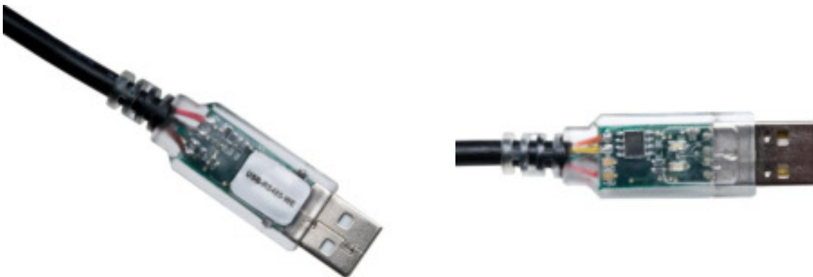
Figure 5.3 USB-RS485-WE Cable images
