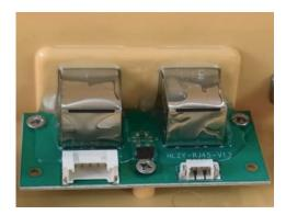
If the battery is installed in a humid environment conducive to condensation, or in a place where rain can reach the battery; please apply dielectric sealant around the RJ45 ports. If you are plugging in an RJ45 cable permanently, then fill the port completely with dielectric grease and then plug in the cable. Be generous, it should overflow.
